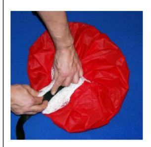
Now quarter the ZeroP fabric to keep the mesh and the bridle inside the handdeployment.
