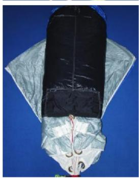
S-fold the lower part inside under the tailpocket.
