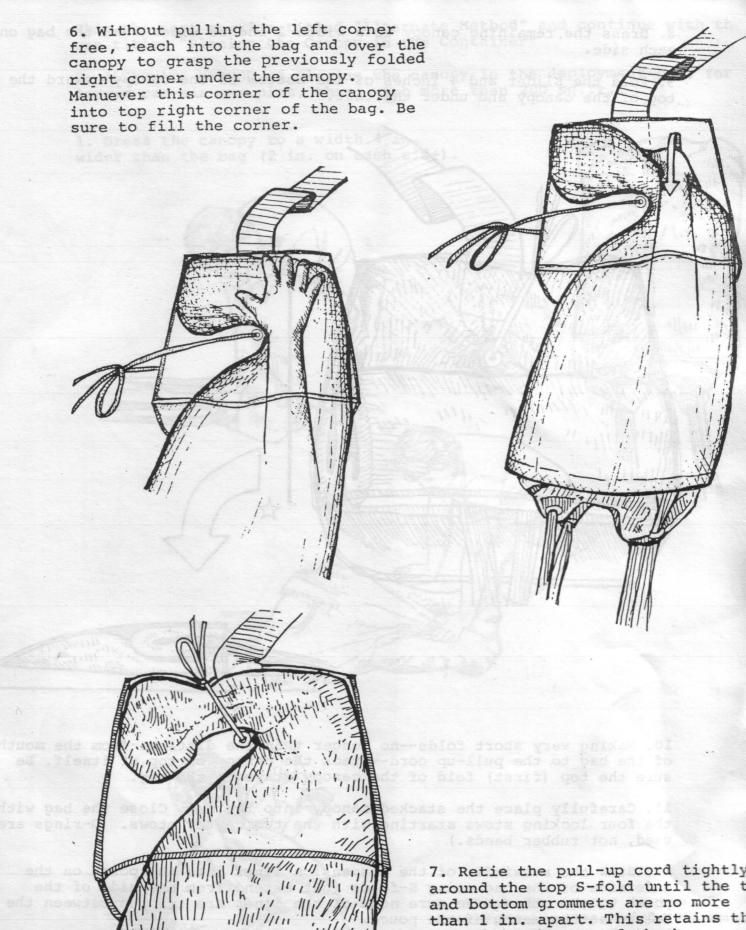
7. Retie the pull-up cord tightly around the top S-fold until the to than 1 in. apart. This retains the S-fold in the top of the bag throughout the rest of the packing procedures.
