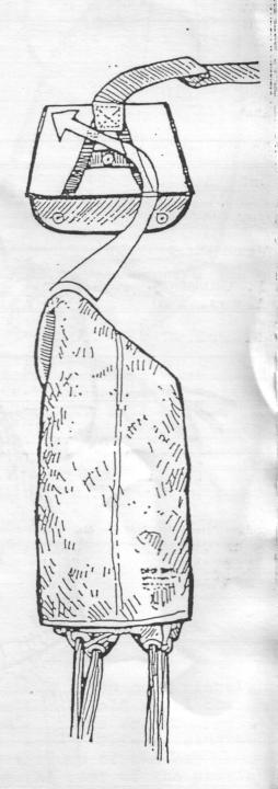
5. Kneeling as before, grasp the top left corner of the flaked canopy and going around to the right of the pull-up cord, place the corner of the canopy into the top left corner of the bag. Be sure to fill the corner.
