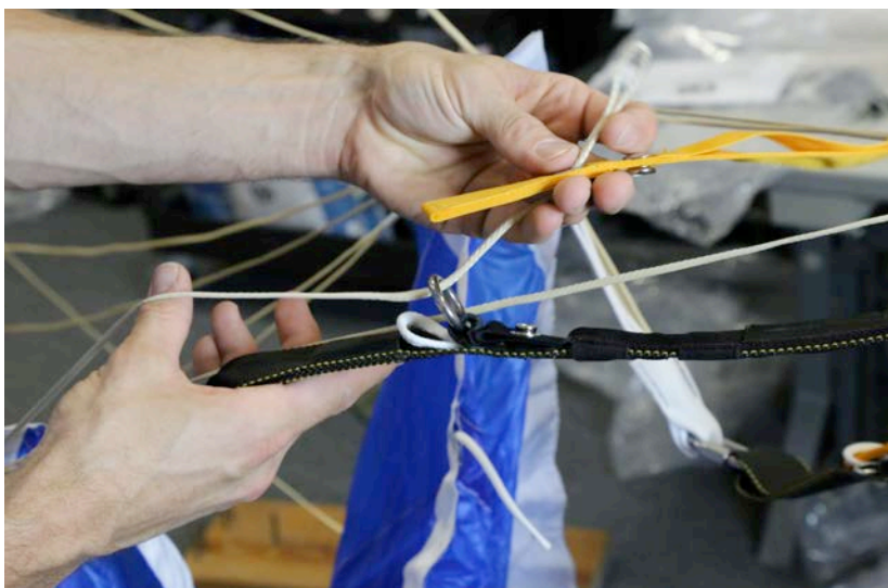
Insert primary control lines through large guide ring, then through primary toggle grommet.
