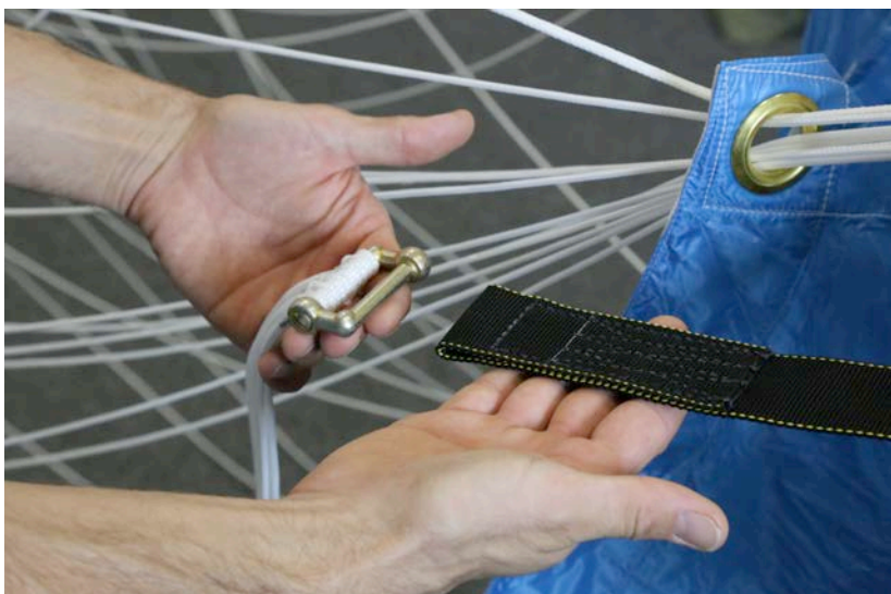
Place and pair reserve riser with correct line group and L-bar
