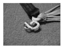
6. Lock running end by pulling ring through loop.
