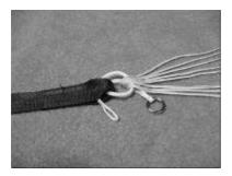
3. Wrap-It<sup>TM</sup> through lines and riser a **second** time...
