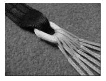
9. Rotate ring into riser and shape link as shown above.
