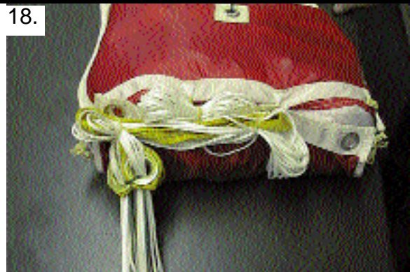
18. Make the third locking stow. Including the remainder of the slider.
