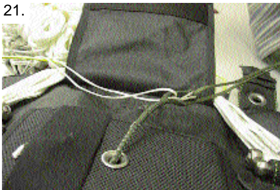
21. Route one pull-up cord through only the green closing loop. Route another pull-up cord through only the white closing loop.
