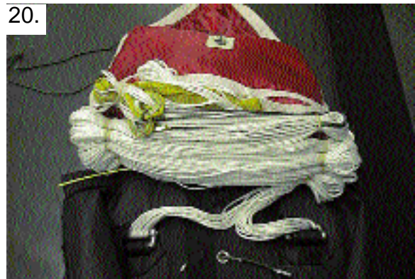
20. SUPERVISOR INSPECTION. Proper d-bag closing and line stowage.
