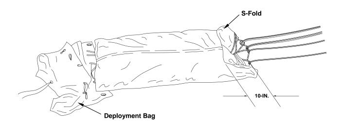
16. Place hand firmly on canopy at suspension line end. Place other hand under canopy approximately 10-inches from end of first S-fold.
