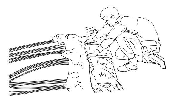
2. Starting with high points on cell 1, pull out seam and smooth cell from leading edge to trailing edge.
