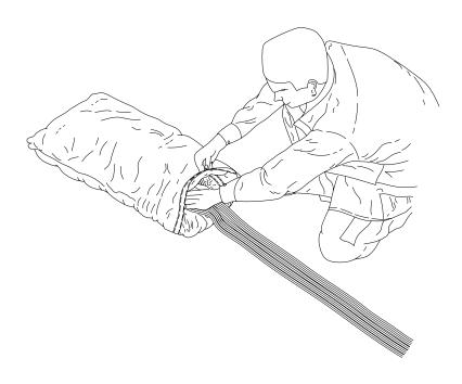
26. Place left hand one deployment bag length up from base of canopy. Grasp upper portion with the right hand. Fold upper canopy over lower canopy.
