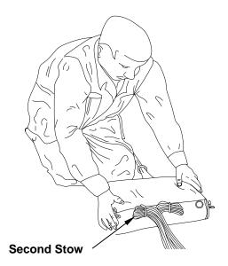
3. Finish locking deployment bag by passing retainer bands through the two outboard grommets, then make third and fourth suspension line locking stows.
