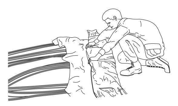
2. Starting with high points on cell 1, pull out seam and smooth cell from leading edge to trailing edge.
