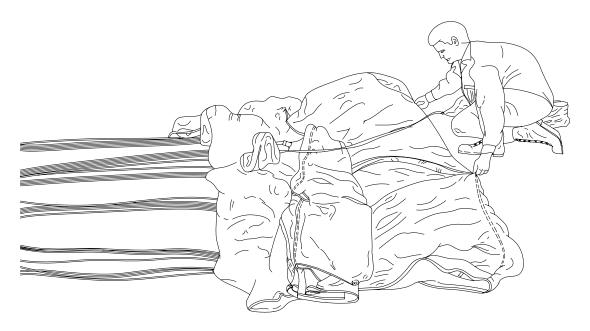
3. Continue to flake canopy by pulling out seams, one by one, on each remaining cell. Smooth each cell until all cells are flaked and all line groups are clearly separated and tight.
