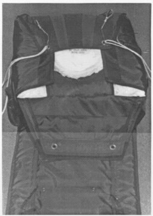
Step 25 Close bottom flap over side flaps and compressed pilot chute and secure with temporary packing pins.
