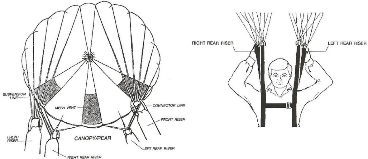
The Preserve I canopy can be turned to the right by pulling down the right steering toggle located behind the right rear riser; the same applies for a left turn. The parachute will continue to turn until the steering toggle is let all the way up to the steering line guide ring.
