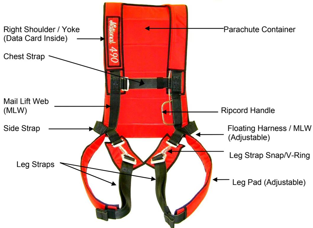
The final adjustments should be comfortable but snug and is determined by a compromise of the sitting and standing positions. Tuck leg strap ends into leg pad cushion and/or stow in keeper. Stow chest strap.
