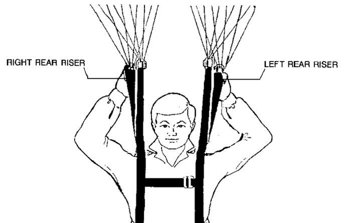
The Parachute can be turned to the right by pulling down the right rear riser 6" to 12", the same applies for a left turn. A rear riser can most effectively be pulled down by placing fingers between suspension lines as they attach to the connector link on the end of the riser. (See diagram above right.) The Parachute will continue turning until the rear riser is released. It takes about 8 - 10 seconds to complete a full 360 degree turn.
