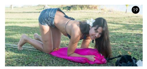
Put one hand or forearm on top of the slider edge of the bundle above the warning label, and the other hand underneath a little farther up, making an S-fold as shown in **photo 20**.
