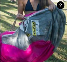
All the lines are now bunched up in the middle, so pull each stabilizer panel out one by one and be sure that none of the lines are wrapped around a slider stop or a stabilizer.
