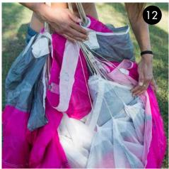
The lines should be in the centre and the fabric towards the outside, as demonstrated in **photo 12**. Check the stabilizers are still clear.
