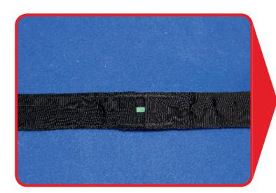
Set the kill line through holding the main bag and pulling the top end of the pilot chute at the same time until the viewing window shows the green marking
