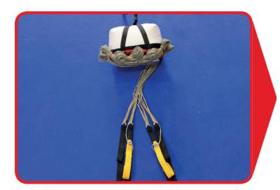
Loop the suspension lines in S-loops and pay attention to leave sufficient overlength. The overlength should be between 15"-20".
