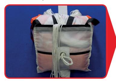
Lock the freebag closed with two loops of suspension line. Only Sife safety stows in the right length should be used, not rubber bands. The locking stows should not be shorter than 2" and not longer than 3". For protecting the reserve suspension lines make sure that the velcro is covered.
