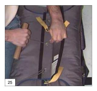
26. Keeping the corners as neat and full as possible, carefully close the corners of the containers as shown. Use your finger to reach inside and poke the corner tuck out if needed.
