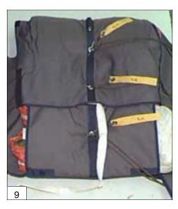
10. Mate the 6" sections of Velcro on the sides of the top flap by pulling the top flap over, down and around the canopy and fastening it to the corresponding Velcro on the pack tray. Leave some of the canopy material sticking out on all four corners – doing so will fill the corners of the container and result in a cleaner looking container when closed. Be sure to keep the bottom flap in position during this procedure.
