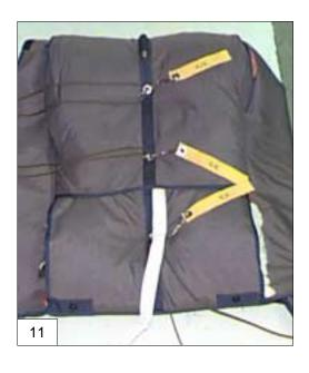
12. "S" fold the pilot chute bridle between the top and center grommets on the top flap.
