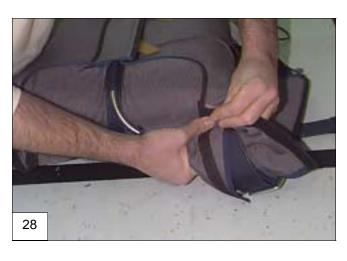
28. Route the ripcord through the housing and replace the temporary pins with the ripcord pins. Remove the pull-up cords being careful not to burn the closing loops. It is recommended that you place the pin between the loop and cord before removing the pull-up cord.
