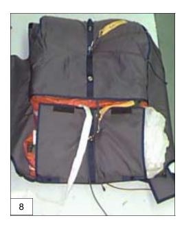
**9.** Mate the top and bottom flap Velcro, routing the pilot chute bridle through the gap between the Velcro segments on the flaps.
