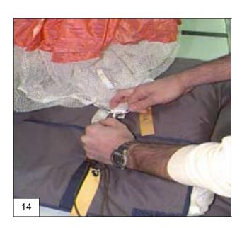
15. Compress the pilot chute and pull all of the material clear of the spring.
