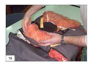
Tuck the folded pilot chute material around the pilot chute crown taking care to support the spring as noted previously.
