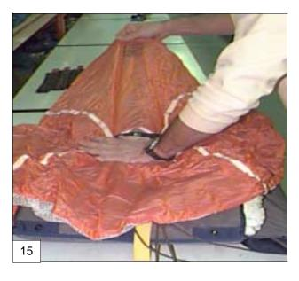
16. Hold the compressed pilot chute in place (your knee works well). Carefully fold the pilot chute material that is covering the bottom of the container and place it against the compressed pilot chute. DO NOT TRAP ANY MATERIAL INSIDE THE PILOT CHUTE SPRING! Pass your pull-up cord through the grommet on the pilot chute crown and pin.
