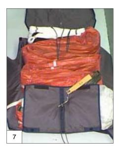
8. Pass the top and center pull-up cords through the grommets in the top flap, fold the flap over the canopy, and hold in place with temporary pins. The top flap will overlap the bottom flap approximately 1".
