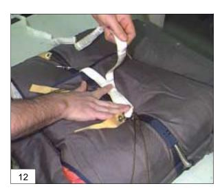
13. Position the pilot chute base on top of the folded, pilot chute bridle, aligning the grommets located on the base of the pilot chute with the top flap grommets. Pass your pull-up cord through the bottom pilot chute grommet and pin the pilot chute in place.
