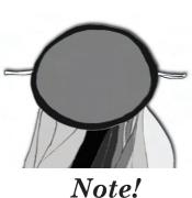
Be careful not to catch pilot chute canopy cloth below stitch line at the top of the pilot chute. Doing so may result in stress being put on the cloth resulting in a hole in canopy.
