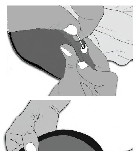
**8.5** Hand tack new cap in place at 90° angles to the loops.
