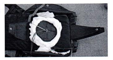
Neaten the pack, seal the ripcord, close the top cover after filling in the data card.
