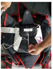
Fold the rest of the bridal above flap #1. Pass the pull up cord cleanly through the pilot chute from bottom
