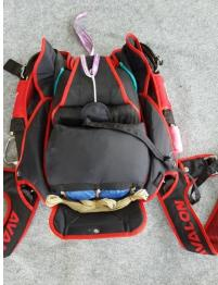
At this stage adjust the closure loop length to suit the main canopy size.
