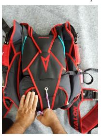
After closing all container flaps insert the closing pin. Make sure the bridal is exiting from the top right
