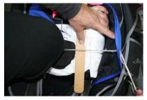
Install the reserve pin through the reserve cable eye. Insert the pin through the closing loop and poke it
