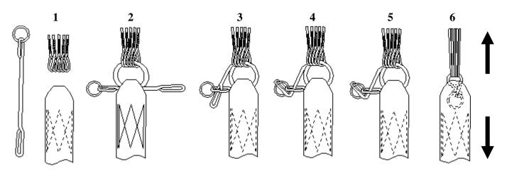
Secure the Soft Link ring in the webbing pocket, and hand tack as shown
