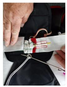
Fold the red marked part of the bridal and poke it into the red marked area. Close flap #2A
