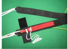
Slide the toggle finger into the pocket. Slow the extra line and close the Velcro. Fix and secure the toggle on the rear riser
