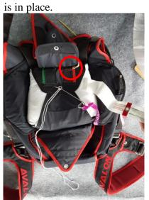
Pass the FORS connection loop trough the lanyard ring.
