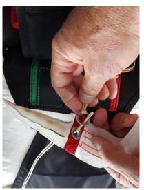
Back the FORS connection loop trough the bridal grommet and secure it with the FORS yellow cable.
