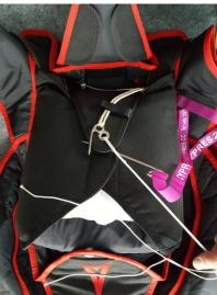
Install the reserve pin through the reserve cable eye. Insert the pin through the closing loop and poke it under the protector pocket. Close the reserve top flap.
