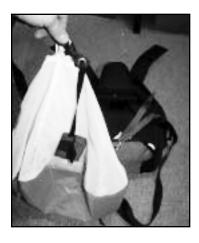
After placing the main canopy in the container, remove all twists in the bridle, and check that the pilot chute is cocked.
