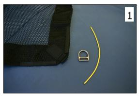
Orient the slider with Type 17 ring retainer and cable channels UP.
