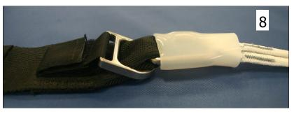
Secure the RAS ring to the riser using the RAS ring keeper attached to the riser. Slide the link cover over the link.
