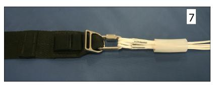
Pass the RAS ring over the link onto the end of the riser.
