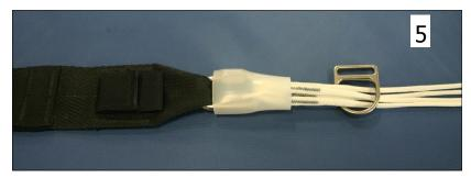
Separate the ring from the slider by removing the yellow cable freeing the ring from the Type 17 retainer.
