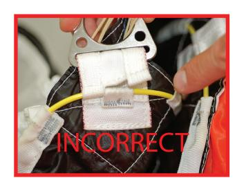
CAUTION!! ENSURE THAT THE YELLOW CABLE GOES THROUGH ALL THREE TAPE LOOPS. The photo to the left shows an incorrect assembly.
