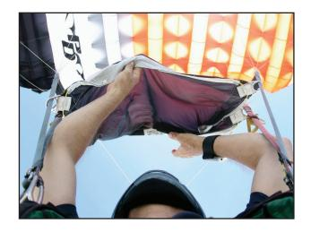
Once you have ensured that the parachute is fully functional, cleared your airspace and pointed the canopy on the desired heading relative to the DZ, locate the leading and trailing edges of the slider in the center of the span (where the release lines are located).
