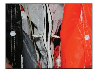
Locate the plastic snaps on the trailing edge of the slider and the snaps on the aft portion of the stabilizer edge.
