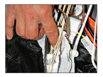
Assure that the control lines stay under the stabilizer and do not cross over the snap.
