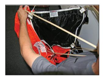
Upon complete assembly of all corners, perform a continuity check of the slider by raising the trailing edge up to show all rings and visually tracing your eyes from corner to corner. Check for proper ring and slider orientation.
