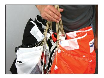
Flake the canopy as you would in a normal pro pack. Make sure to quarter the slider well up against the bottom skin. Ensure that all slider rings are well seated against the stops and that the RDS lanyard is freely routed towards the tail of the canopy.
