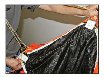
Carefully trace down the left edge of the slider towards the front left corner and attach the next ring in the same careful manner as before. Ensure that the slider edge is not flipped and appears correctly as shown.
