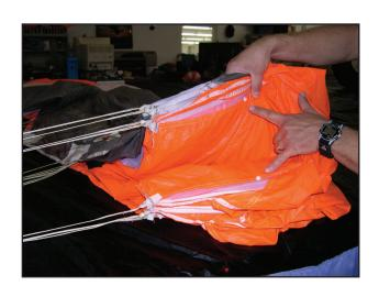
This canopy is equipped with plastic snaps that help secure the slider to the canopy during packing. Two snaps are located on the leading edge tape of the center cell.
