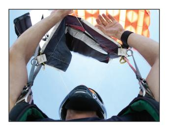
Pull the two release lines simultaneously forward or backward. (Forward shown in photo)
