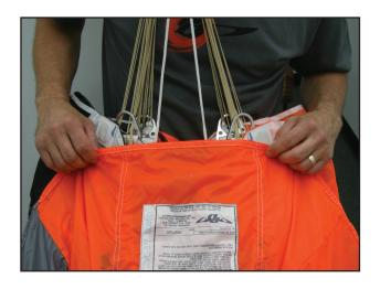
Run the lanyard and d-bag over the shoulder while completing the preparation of the canopy and wrapping up the tail during the pro pack.
