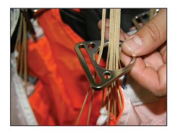
Grasp the left rear ring in the left hand as shown; be aware that the lines must run cleanly thru the ring.
