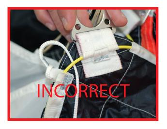
CAUTION!! DO NOT ALLOW THE LANYARD TO GET TRAPPED UNDER THE YELLOW CABLE. The photo to the left shows an incorrect routing.
