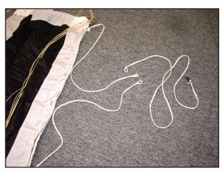
Next, remove the longer length of line in the lanyard assembly by undoing the larks head at the point where the lanyard junctions into two lines.
