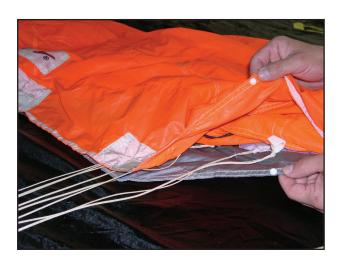
Two other snaps are located on the stabilizer perimeter tape, just aft of the C-line attachment points.
