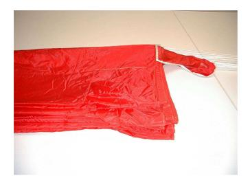
Fig. 10 Placing the Folded Gores
