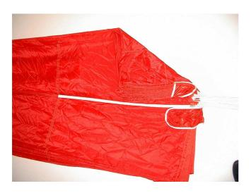
**Fig. 14**Folding Lower Lateral Bands on the Right
