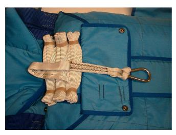
Fig. 5 man./aut. Stowing the Static Line
