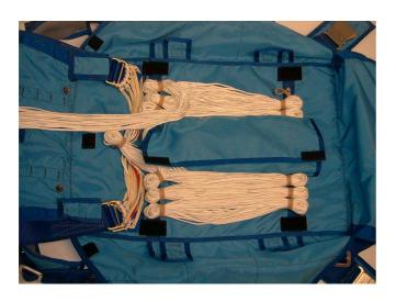
Fig. 18 Stowing the Suspension Lines
