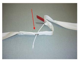
"Arm" the M.A.R.D. "Reserve Boost" at this time by feeding the Spectra Line Loop down through the #0 grommet of the Reserve Free-bag Bridle.
