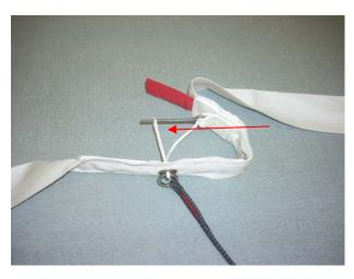
Slide the Long Pin through the loop then stow into the channel under the tuck tab flap. Be certain that it is in it's own channel.
