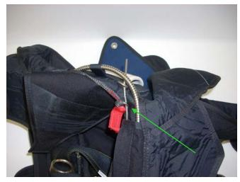
Be certain that the Reserve Ripcord Cable passes through the guide ring then under the cutaway housing as shown above.
