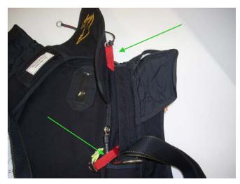
Close the cover of the RSL channel. Be sure there is enough lanyard to connect the clasp to the ring on the Main Risers. Extra lanyard can be left at the top end of the channel.
