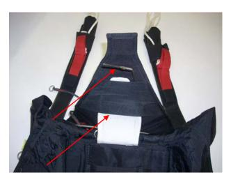
Before proceeding check to be sure that the Top Closing Flap and the Ripcord is under the tape of the Top Cover Flap.
