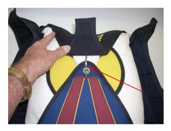
Close and secure the Bottom Closing Flap with the Reserve Ripcord Pin.
