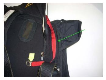
Mate the Pile Velcro of the "Reserve Boost" RSL with the Hook Velcro under the Left Side of the Shoulder Yoke.
