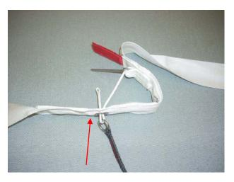
Loop the Spectra Line back up through the #0 grommet of the bridle.
