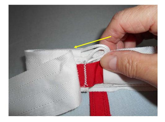
Stow any excess Spectra line into the pocket shown.
