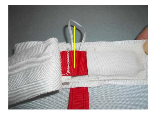
Pull any excess Spectra line up through the grommet.
