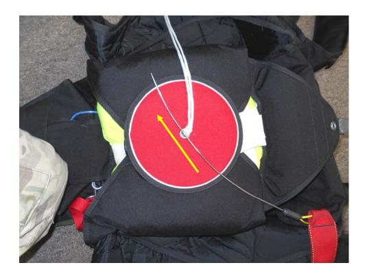
Secure the Reserve Pilot-chute with a temporary pin.
