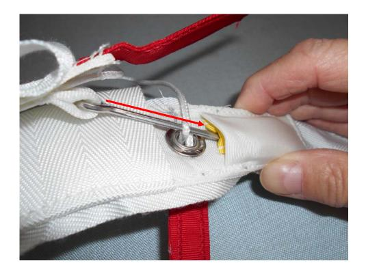
Stow the long pin into the channel under the tuck tab flap. Be certain that it is in it's own channel of T-III tape (yellow).
