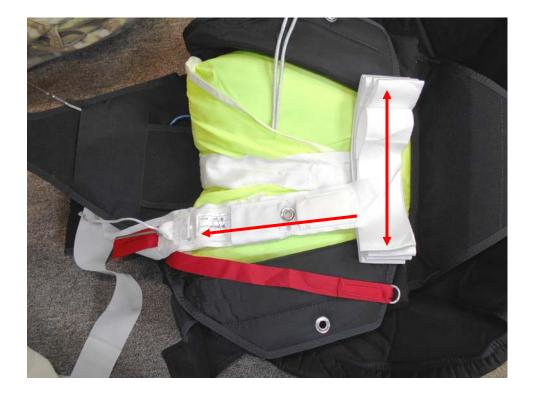
"S"-fold the bridle into 6"-8" folds across the bottom of the Free-bag to the M.A.R.D. "**Reserve Boost**" Modification.
