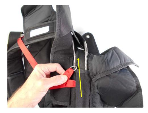
Pass the Ripcord Pin and Cable through the ring on the RSL.
