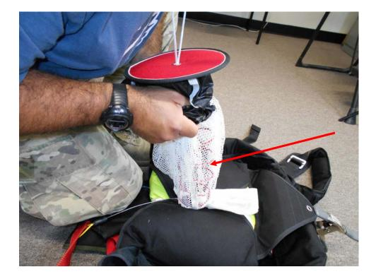
Thread the pull-up cord through the Reserve Pilotchute and center over the side flap grommets.
