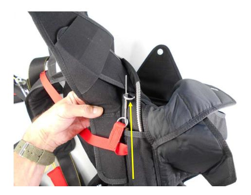
Pass the Ripcord Pin and Cable through the guide ring on the *Wings* Container.
