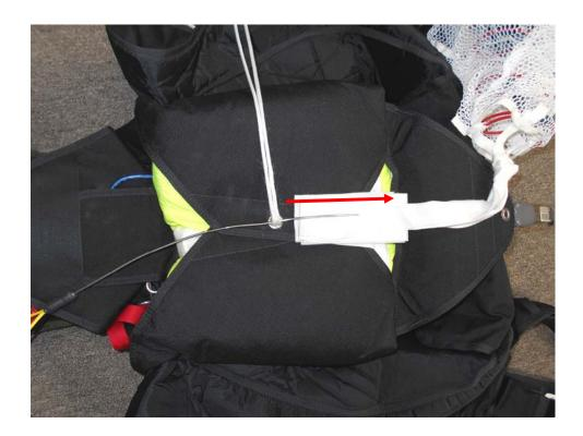
"S"-fold the remaining bridle at a right angle to the tucked bridle and secure with the temporary pin.
