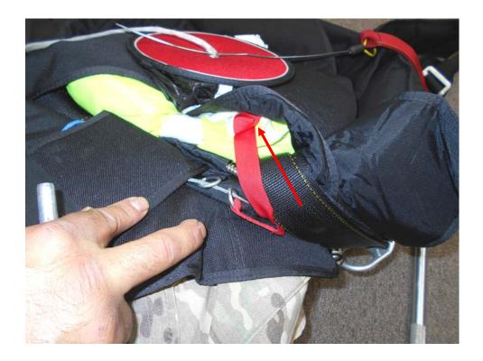
Tuckanyexcess**"ReserveBoost"**lanyard into the pocketon the Free-bag.
