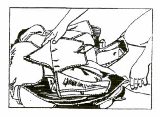
3. S-fold the length of free bridle onto the top of #2 flap up to the base of the pilot chute.
