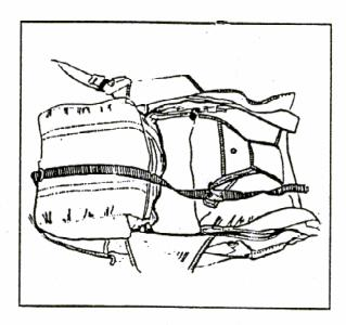
7. Follow the risers from the harness rings and lay them flat along the sides of the container. Distribute the connector links along the sides of the packtray. Route suspension lines neatly.
