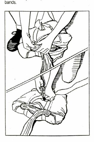
2. Stow the remainder of the suspension lines into the pouch on the underside of the bag using s-folds that extend from one side of the bag to the other.
