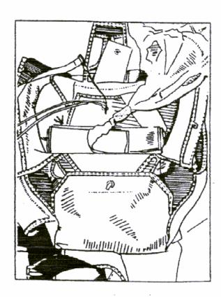
NOTE: When packing the *Centaurus* equipped with a Molar freebag, place several short folds of bridle between the freebag grommet and the top of bag in order to fill in the "valley" between the ears of the Molar freebag. Close the reserve no. 1 flap over these folds. With the no. 1 & no. 2 flaps closed, the orange assistor pockets should be visible. Fold the remaining bridle to form a "V" with the point towards the main container.
