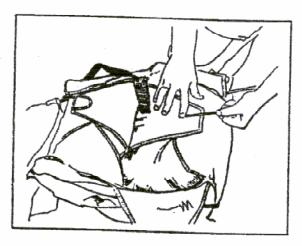
Thread the pull-up cord through the right flap.Pull and pat until the loop comes through the grommet. Hold in place with your knee.
