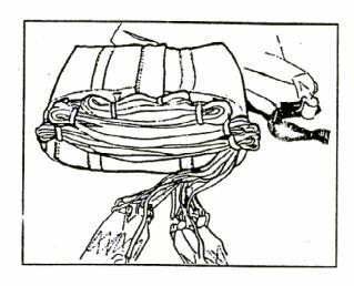
and place it in the main container, grommet side up and mouth side down. Rotate the bag out of the way.
