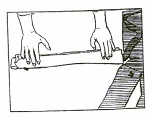
7. Fold pilot chute to half its length, skirt to handle.
