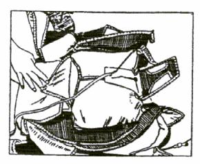
11. Replace the temporary pin with the reserve pin, routing the cable through the RSL ring. The end of the pin slides into the channel in the bottom flap.
