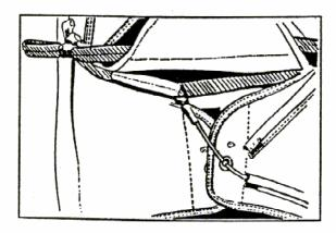
4. Triple stow the first fold of static line in the rubber stow band. It is important to triple stow in order to prevent the drag on the static line from prematurely pulling the cable free and opening the container. 5. Close the container flap and stow the remaining static line from left to right across the container. The static line snap can be dipped to the cable housing until ready for use.
