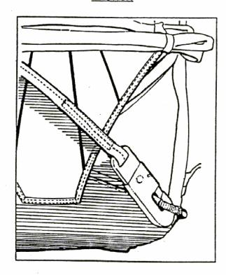
Check the condition of all components frequently. Direct bag static line deployment can subject the D-bag, static line, and other parts to stress and wear. Replace any components that show signs of damage.
