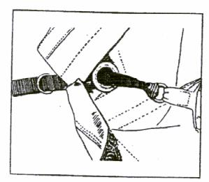
The stop ring on the bridle lies between the deployment bag and the pilot chute.
