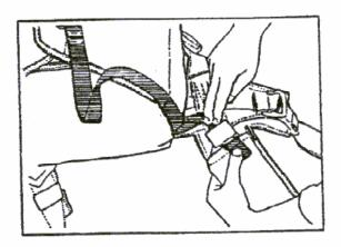
Mate the velcro on bridle to the harness velcro. Tuck excess under the bottom of the right flap.
