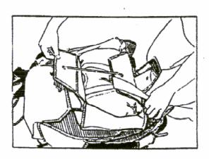
Exerting even pressure, push both flaps together so that they center over the grommet of the reserve bag. Pull up smoothly on locking loop and secure with temporary pin.
