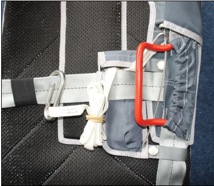
Photo No. 6. The static line with the release handle ready for use.
