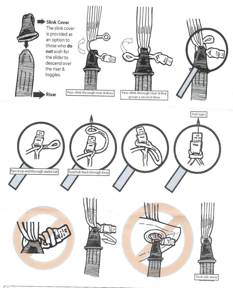
During the first 15-20 deployments on a set of slinks they will develop a "set". Make sure this set happens properly by keeping the Slink tab positioned inside the riser during these initial pack jobs/deployments. MAN-016-D REV. C
