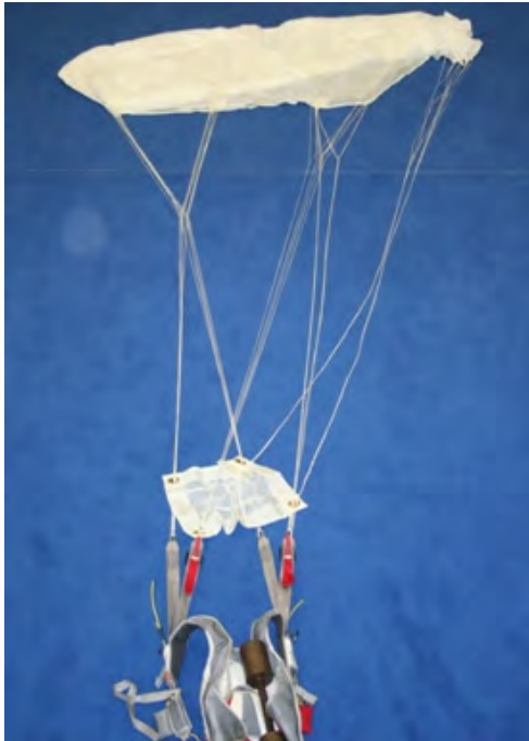
Step 1 Lay out the parachute and sort the lines.
