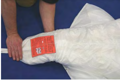
Step 12 Narrow down the base of the canopy even more to be able to grasp it with one hand.
