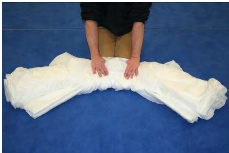
Step 14 Spread the canopy down the centre and start reefing up the centre cell. Make sure to kneel on the base S-fold to keep it securely in place.
