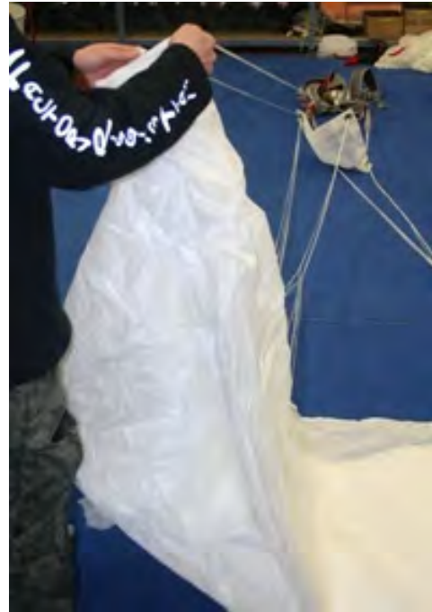
Step 2 Perform a line check by making sure the steering lines run free through the sliders grommets to the steering toggles.
