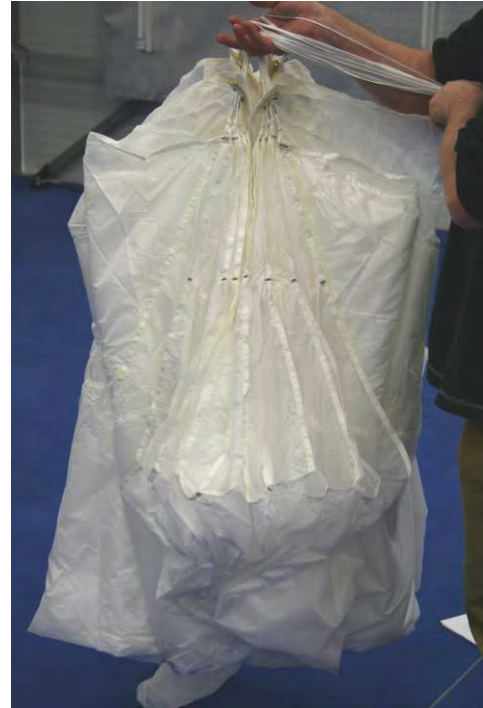
Step 6 / 4 Correctly folded canopy shown from leading edge side.
