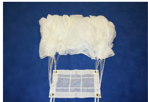
Step 4 Prepare the canopy for packing by moving the slider up to the base of the canopy.
