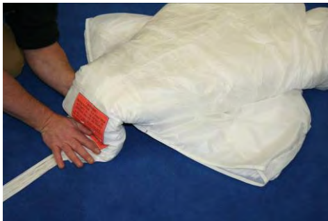
Step 13 / 1 Perform a S-fold backwards towards the line strand.
