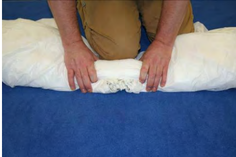
Step 16 Roll the centre cell forward and on top of the base S-fold.
