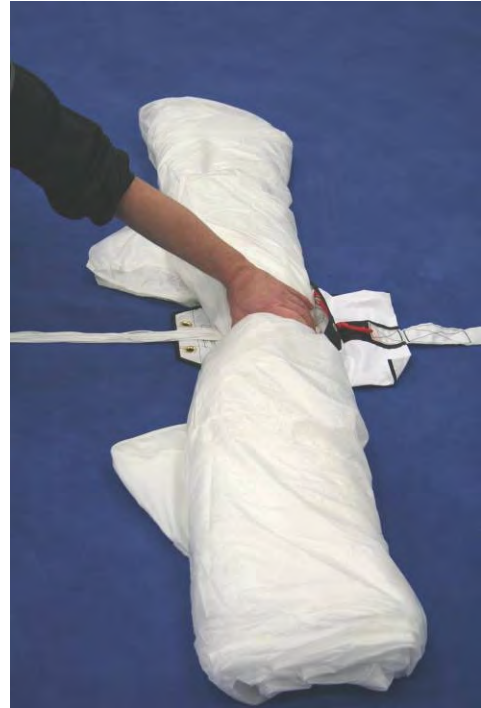
Step 17 By doing as described in Step 16, you receive a configuration as shown in this picture. This will allow you to grab the very small base of the pack job and be able to lift it up to position the reserve bag right underneath the base. The base goes in the bag first and stays nice and unaltered.
