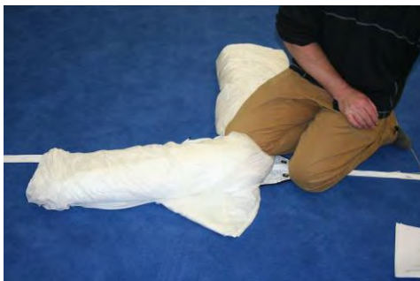
Step 18 Slide the left ear 90° forward while still kneeling on the base.
