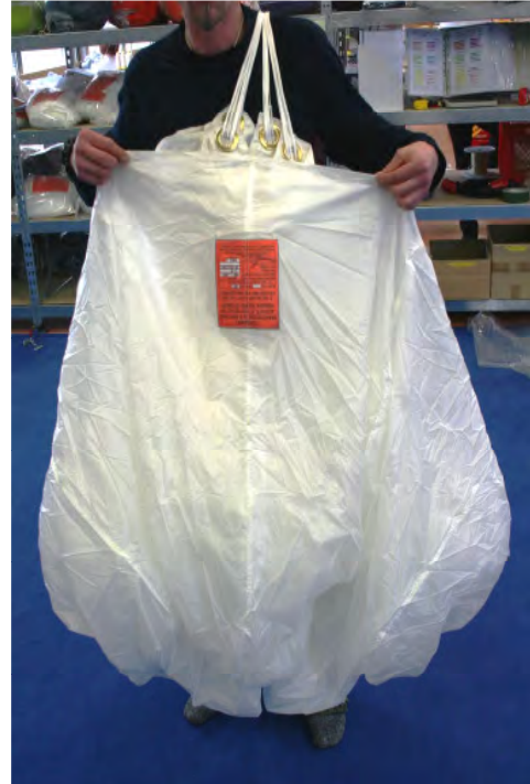
Step 8 / 1 Pull up the centre cell with the trailing edge and position it just above the slider grommets and around the line strand. See details on next picture.
