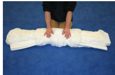
Step 15 Dressing the centre cell in it's reefed configuration.
