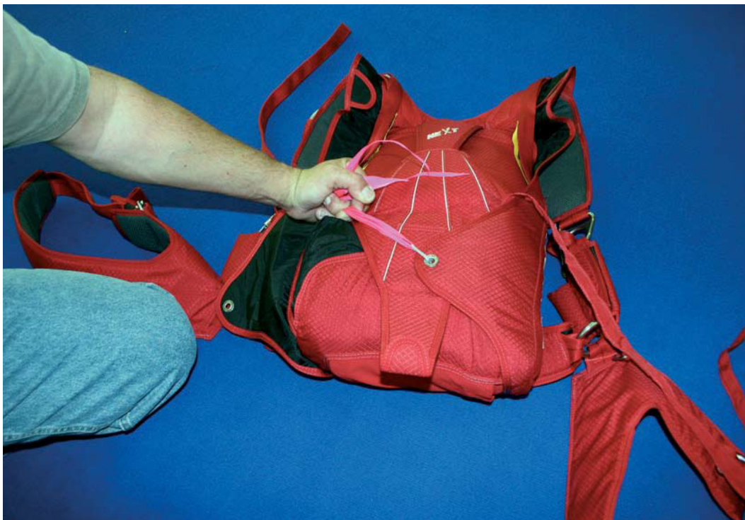
Picture 23 Very important: Close the right flap first. This assures the symmetry of the side flaps with the pin cover flap.
