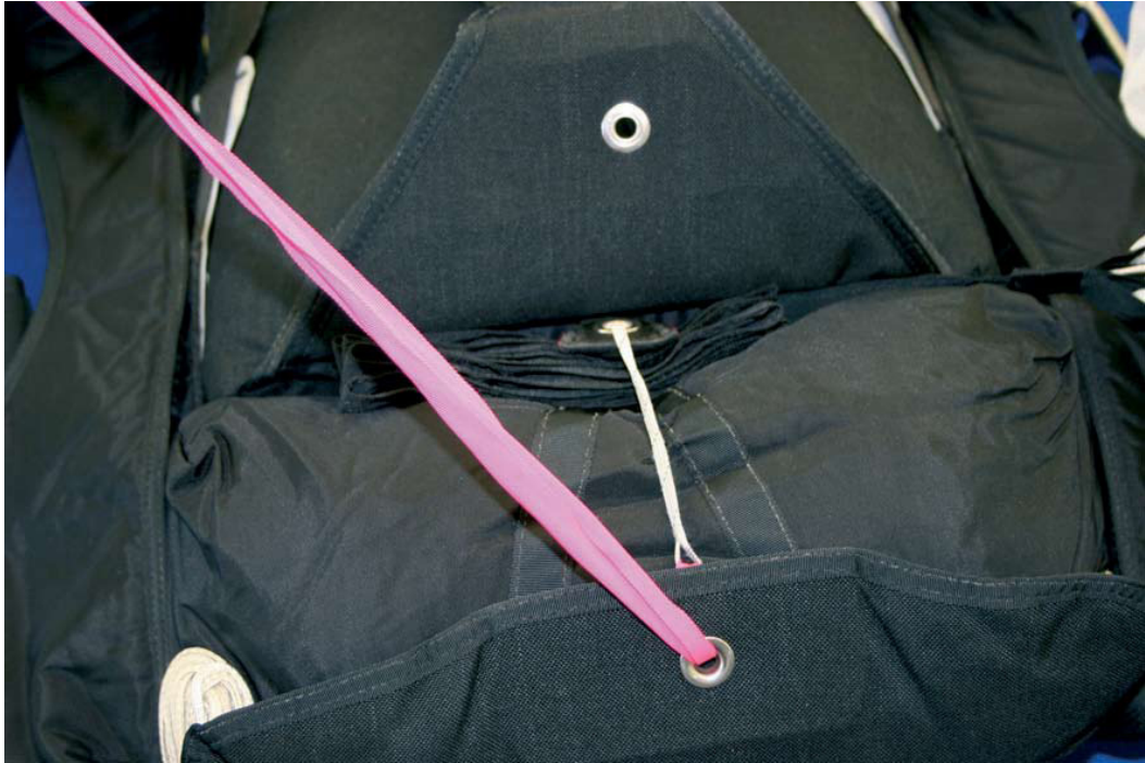
Picture 41 Close flap # 1. This will assure that the bridle will be kept safe in position.
