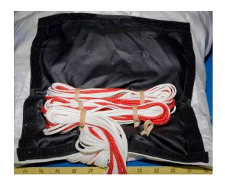
**5)** Leave approximately 12"-14" of line unstowed between the connector links and the mouth of the tail pocket.
