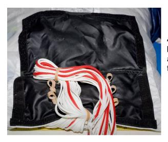
**4)** Begin stowing the remaining lines in the rubber bands on the tail pocket, starting with the bands at the <u>top</u> of the tail pocket (farthest away from the tail seam).
