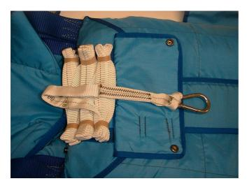
**Fig. 5** man./aut. Stowing the Static Line
