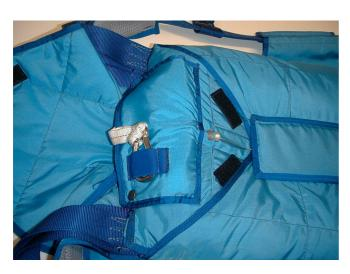
Fig. 6 man./aut. Stowing the Snap Hook
