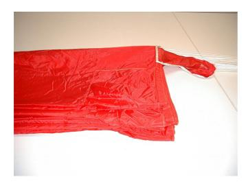
Fig. 10 Placing the Folded Gores
