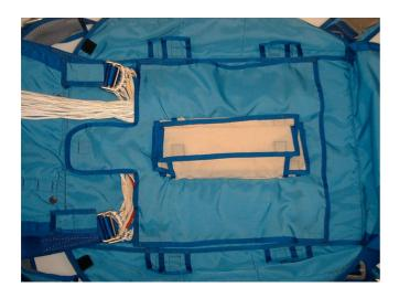
Fig. 19 Covering the Suspension Lines
