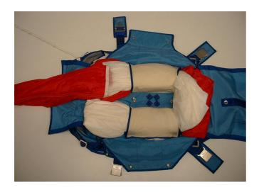
Fig. 22 RE-5L Series 5 Making the Second Fold
