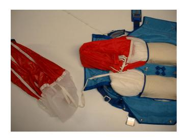
Fig. 23 RE-5L Series 5 Folding the Apex
