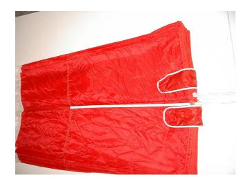
**Fig. 13** Placing the Skirt Retainers
