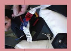
Fit the red line on to the metal Skyhook under the clear Plastic and seal with one turn red riggers thread through the small hole in the plastic.
