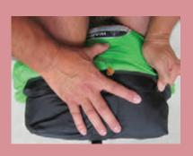
Roll the parchute down and pull the mouth of the bag out as shown.
