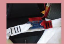
Insert a rifle rod and pull the pull up through the reserve pilot chute.
