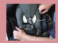
Remove the pull up cord carefully and seal with riggers thread and lead seal.
