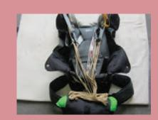
Stack the risers side by side and stow the lines neatly down the sides of the container as shown.
