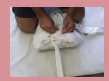
Place a +- 40cm looped Velcro tape with a warning tag attached in the opened line stowage pocket and fit the Velcro together. This is done to protect the lines while been stowed.
