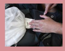
Roll / Fold the material of the pilot chute neatly and fold it on top of the S - folded bridle.
