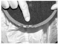
Make sure the overlap on the pilot chute binding is positioned to the top of the reserve container. Slowly compress the spring down. Clear the fabric and mesh from the spring as you compress it.
