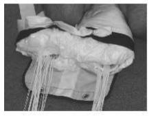
Spread the slider grommets and equalize the pack job on both sides of the freebag.
