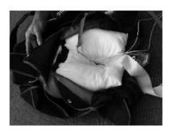
Pull on the pull up cord and pin the closing loop in place.
