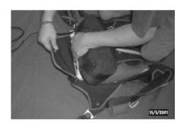
Keep the loop clear while placing the bag into the container
