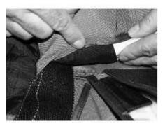
Push the tuck tab on flap number 1 underneath the freebag.
