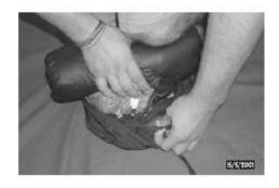
Rotate the parachute forward into the bag.
