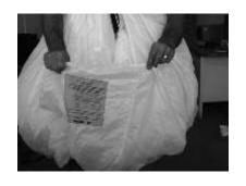
Bring the center of the tail up and over the grommets of the slider.
