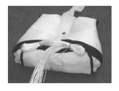
Pull equal tension on both line groups and close the mouth of the free bag using 1.5 inch bites thru the shock cord elastic on each side.
