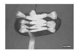
Complete the line stows using one and half inch bites.
