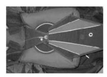
Insert the Ripcord Pin. Carefully remove the pull up cord. Use the packing paddle to tidy your pack job.
