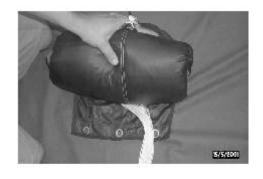
Rotate the parachute slightly and place on the flap as shown.
