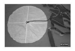
Lay the pilot chute out as shown. Note the position relative to the container.
