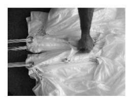
Pull the slider up against the slider stops and quarter it.
