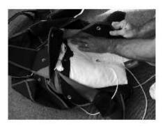
Make sure you push the corners of the freebag all the way into the bottom corners of the reserve container. The two locking line stows should be pushed into position and covered by the protection flap.
