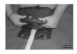
Aggressively rotate the top of the deployment bag towards the floor, whilst trapping the bag between your knees and hands.
