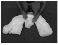
Split the canopy in the center and share the center cell equally on both sides while making bunny ears.
