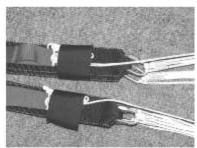
Separate the line groups as per our diagram and walk the lines up to the canopy. Place a weight on the container to get good and even line tension.
