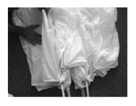
Clear the stabilisers on both sides without disturbing the lines.
