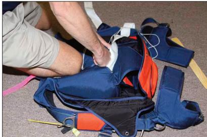
Freebag should be seated all the way to the bottom of the container.
