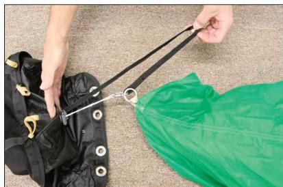
This picture represents the inside of the deployment bag. The Rapide link should be on this side.
