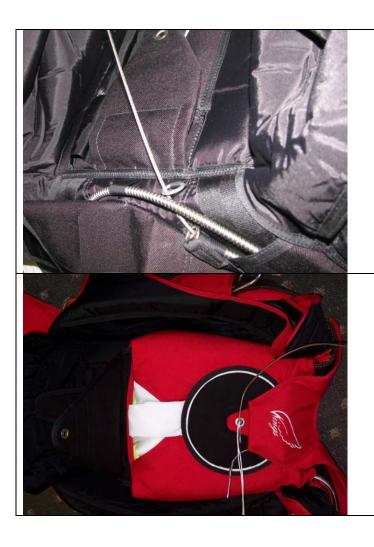
Check the routing of the reserve ripcord. After the end of the ripcord housing, the ripcord should pass through the RSL ring, if an RSL is used, under the cutaway cable housing and through the RSL guide ring. After this, route the reserve ripcord and reserve top flap under the #3 flap 3" wide tape.
