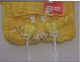
With the tail section flaked, fold the lower third of the parachute on top of itself. For smaller sized reserves, this step may be unnecessary. Also, separate the grommets approximately 6" apart. This will help create a space for the AAD during closing.
