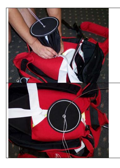
Thread the pull up cord through the base of the pilot chute and through the grommet of the pilot chute cap, without threading through any other components. Compress the pilot chute, making sure to contain all of the pilot chute material between the coils of the spring. Once compressed, pull the closing loop through the grommet of the pilot chute cap and temporary pin the pilot chute in place.
