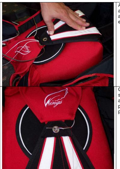
After closing the top flap, the center flap and top flap grommets should almost meet. If the grommets are more than  $1 \frac{1}{2}$ " -2" apart, it could be an indication of too much material in the center of the free bag and not enough in the ears.
