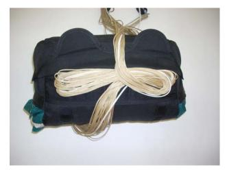
"S-fold" the lines back and forth placing onto the pouch. Leave about 18" unstowed.
