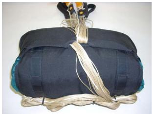
The Deployment Bag is ready to be placed into the Main Container.
