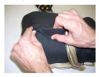
Close the Pouch and tuck the flaps under to secure the lines.
