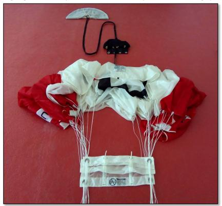
Perform a line check, to see that the line sets are straight, without twists, that brake lines are straight and on the top of other lines, check the continuity above and below the slider.
