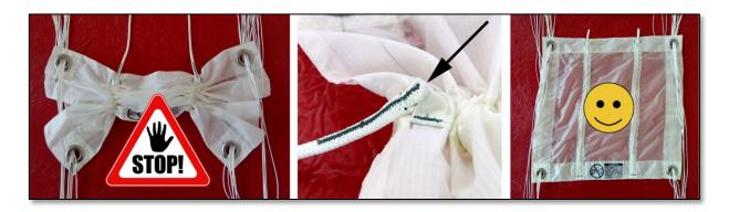
To set the brakes for both steering lines pull the steering line loop through the guide ring on the riser.
