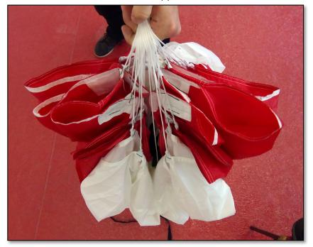
This is a front view of the folded and flaked canopy. While keeping the nose pointed towards yourself, check that the slider is properly positioned and spread between the 4 line groups (front &, back, right & left) and that the slider grommets are pushed all the way up against the slider stops.
