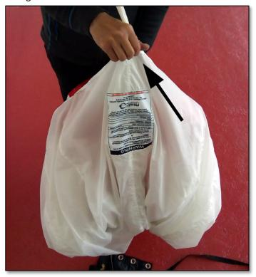
Take both sides of the canopy tail and bring them around towards the front (nose) of the canopy. It is very important to make sure that no (steering) lines pass in front of the leading edge (nose), as this may cause a line-over malfunction.
