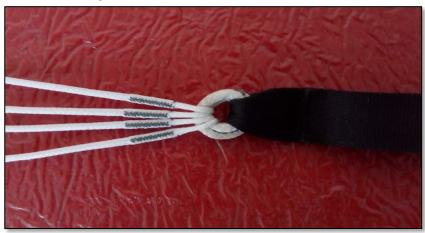
If you are using steel (French) links, finger-tighten the nut as much as possible, and then apply ¼ up to ½ turn with a wrench. Do not over tighten as this can damage the thread or crack the link nut, causing the link to fail. Pull the slider bumpers (covers) over the links to protect the lines.
