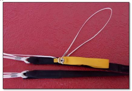
Stow the slack brake line on the riser.
