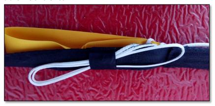
Brake set and secured for packing/jump.
