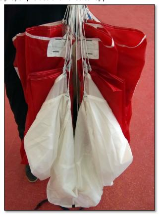
Pick up the centre cell by its trailing edge (identified by small red or black tape) and lay it on top of the lines just below the slider.
