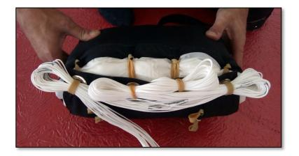
When stowing the lines, we are recommending to leave between 50 - 60 cm (20" TO 24") of lines free at the end in order to prevent line twists during opening.
