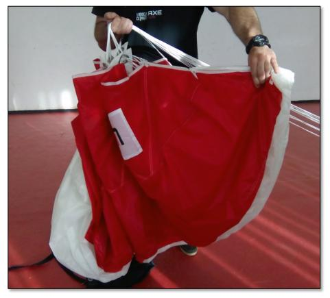
Then, on one side of the canopy, put your hand inside the canopy and make a fold to separate line groups A & B.
