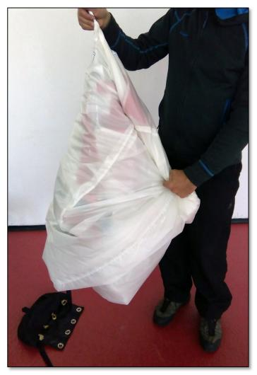
Gently swing the canopy out and lay it on the floor as shown. Carefully push the air out of the canopy. Again, make sure that the slider stays in place against the slider stops. WARNING: IF THE SLIDER IS NOT ALL THE WAY UP AGAINST THE SLIDER STOPS, THE POSSIBILITY OF A HARD OPENING IS SIGNIFICANTLY INCREASED.
