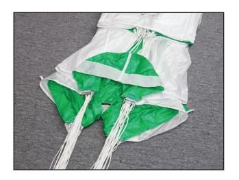
IMPORTANT: Ensure the D-Rings are not twisted. Rotate D-rings (if necessary) around their respective line groups so that the D-ring bartacks on the fabric side of the slider are visible, facing up. The slider warning label will be visible as depicted.
