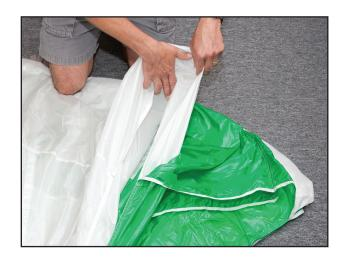
Tuck the overhanging portion of each cell back inside the cell itself. Next, roll the outer three cells on each side in toward the center cell.
