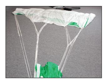
Make a fold of the resultant leading edge so it faces aft, as depicted. This nose configuration helps to reduce opening shock forces, and helps increase consistently onheading openings.
