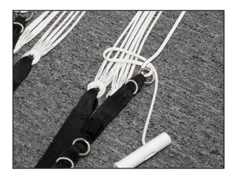
C) Take the loop inboard, going behind (under) the steering line,
