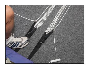
A) Pull steering lines down until the marks line up with riser stop rings.
