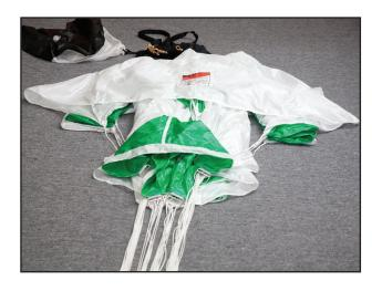
The slider D-rings should seat against the A-flare and stabilizer C-line stops.
