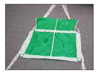
First, unsnap the pocket flap. Spread out the pocket to facilitate pulling the slider up the suspension lines.
