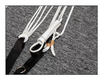
F) Stow the excess steering line in an elastic band attached to the rear riser link. This will further secure the toggle to the rear riser and help prevent it from coming free during deployment.
