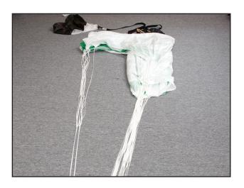
Finally, grasp the "D" line group and place it on top the A/B/C stack, while flaking the material between the two groups to the side. Arrange the S-fold as in previous step. Keep tension on the line groups.
