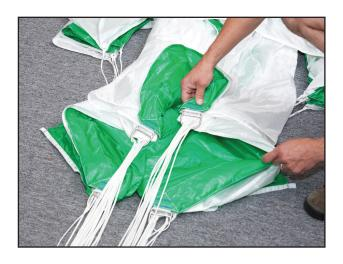
Dress the slider as before, keeping the bottom D-rings snug against their stops, the pocket flap pulled up and fanned out, underneath the canopy.
