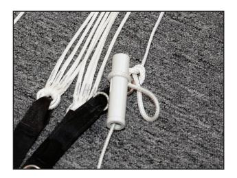
F) Insert the top of the toggle through the remaining loop (it should be snug).
