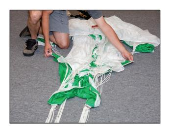
Holding the pocket flap by the corners (grasp the snap tabs), pull the slider up the suspension lines until the bottom (leading edge) D-rings are seated against their respective stops. The pocket flap should be fanned out under the lines and the lower portion of the canopy with no twists, pockets facing down.
