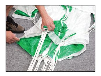
Tip: Lift the upper/trailing edge D-rings to separate line groups and facilitate tucking the sides of the slider into their corresponding locations on the inside of the stabilizer.
