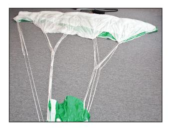
We recommend side-packing your Zero. Lay the parachute on a clean surface and flake it out as shown. No lines should cross each other and the slider should be properly oriented, with steering lines passing freely from the trailing edge through the rear D-rings to the risers. If you are not sure about the continuity of your lines, have a qualified rigger check it.
